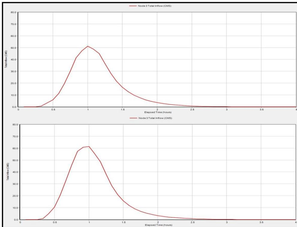
**Figure 9.** Flood hydrograph at Mehmet Oğuz boulevard junction in 2013 (Upper panel) and 2019 (Lower panel).
