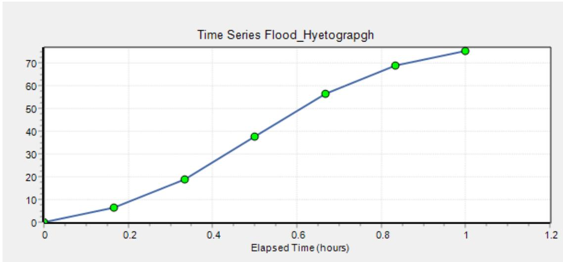
**Figure 3.** 25-year cumulative storm hyetograph having with 1-hour duration.
