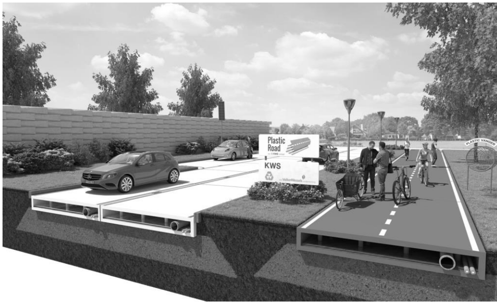
Figure 4: A Plastic Road in Netherlands Made From Recycled Plastic Material (URL-9)
