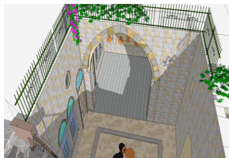
Figure 2. Al Hato dwelling, Gaza old town. 3D AutoCAD drawing showing its architectural elements: courtyard, arches and iwan [Architecture students drafting and rendering supervised by Dr. Abdurrahman Moahmed]
