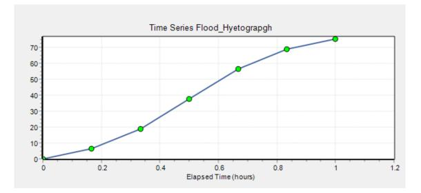
Figure 3. 25-year cumulative storm hyetograph having with 1-hour duration.
