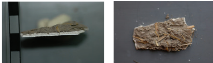
Figure 23. Scaled photo of mud plaster and lime plaster as two layers
